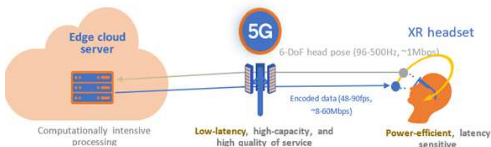
Figure 14: Split XR architecture with M2R2P latency = 5G RTT + Device processing + Server Processing
